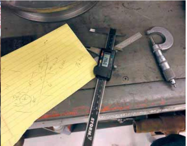
**Precise measurements of the damaged bulkhead were taken and logged into the 3D software so a new part could be produced with a numerically controlled machine.**
