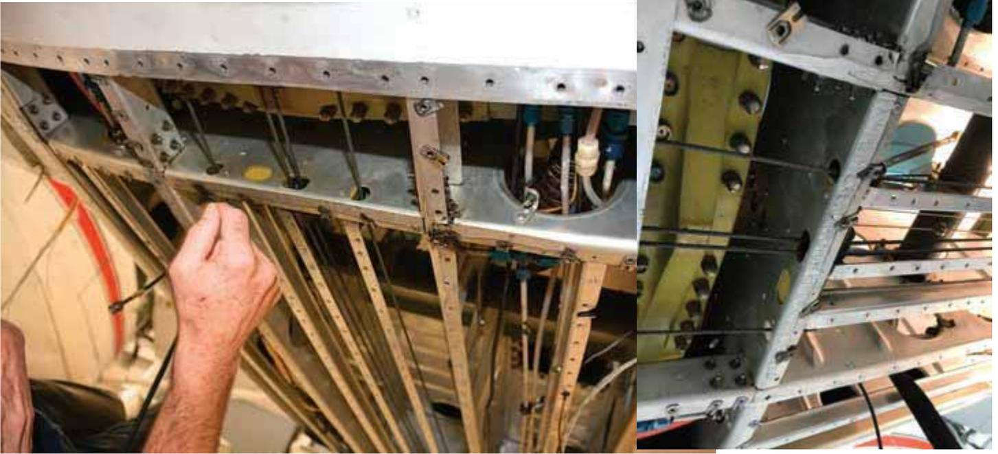
**The bulkhead near mid-fuselage was damaged in the belly landing. Replacing it would have been expensive so a support bracket was designed, milled, and heat treated to provide additional support.**
