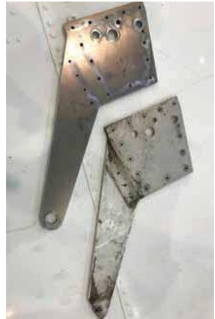
**Flap hinges would take at least six months to get from Beechcraft. To speed repairs, identical replacements were produced using 3D software and a numerically controlled machine.**
