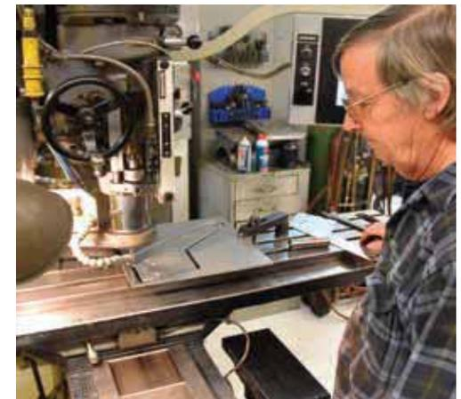
**An old but very precise Bridgeport milling machine with computerized controls was used to produce the replacement flap hinges.**
